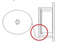
Feed the cut edge of paper into the mechanism and operate the paper feed button
