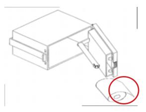
Cut off the end of the paper cleanly with scissors
