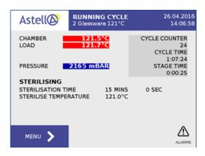
This stage is the main sterilisation process. The stage timing is controlled by the selected temperature probes and the temperature by the pressure set-point. The stage continues for set sterilisation time.
