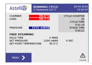
The chamber temperature will stabilise and slowly rise typically 97-103°C depending on altitude and the boiling point of water. After free steam time ends, the system goes to heat to sterilize stage.
