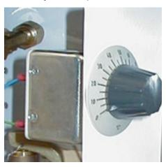
Typical view of cooling lock thermostat
